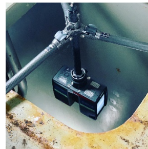
Figure 2: FARO S150 Deployed on LNG Vessel (Inverted and down opening)
