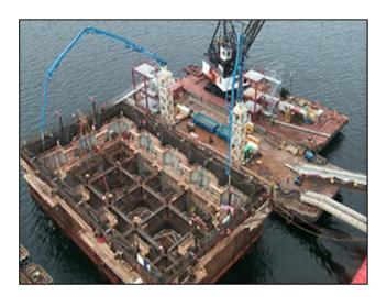
**Catamaran Barge:** Designed for various applications with up to 4 lifting lugs on the cross beams. Capacities up to 4000 Tons. Design and analysis of cross beams and the barges. Structural analysis, stability and ballasting, motions analysis, and mooring analysis.
