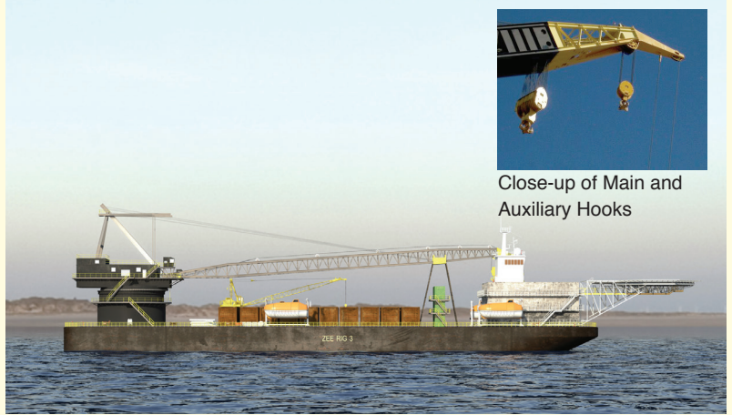
Side view showing 275 Ft. (83.8m) boom of AmClyde Marine Crane
