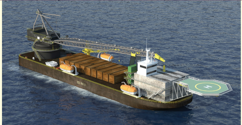
Zee Rig 3 shown with AmClyde Model 52 Marine Crane and 275 Ft. (83.8m) Boom.
